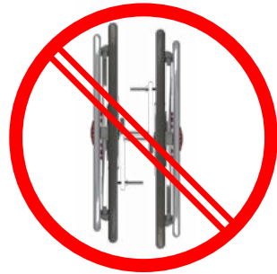
AXLES FACING IN INCORRECT
